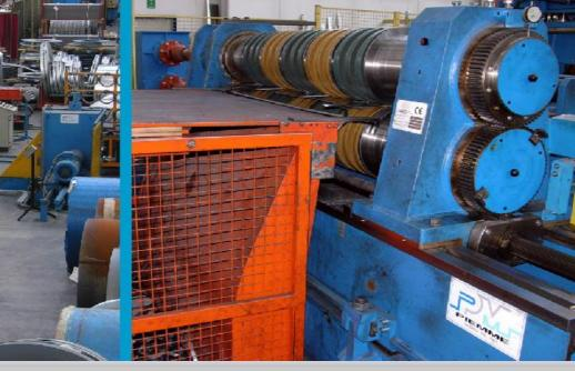
View of line and detail of shear w. circular blade
